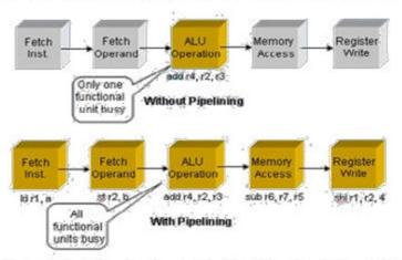
instructions are being processed simultaneously. An implied assumption in this case is that at the end of each stage, we have some sort of a storage place (like temporary registers) to hold the results of the present stage till they are used by the next stage.
